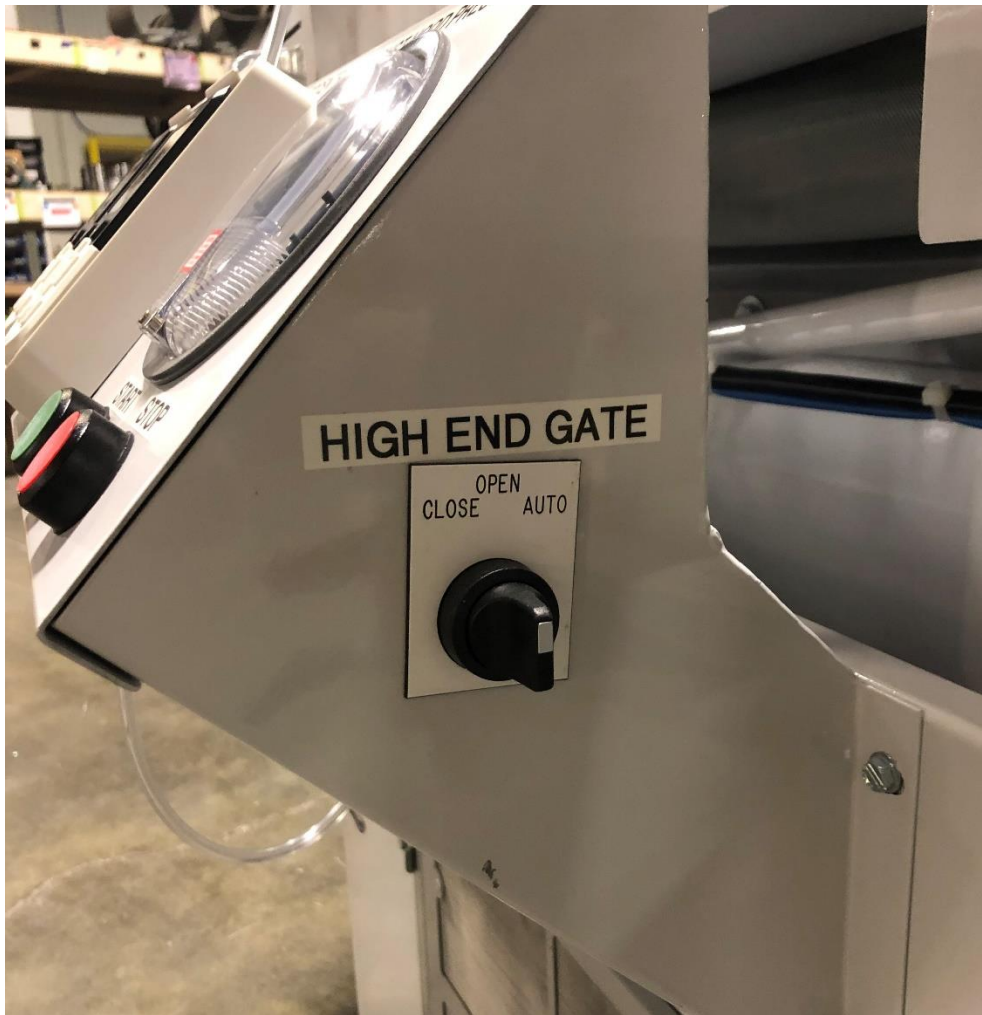
FIGURE 10: GATE 3-WAY SWITCH ON THE CONSOLE
