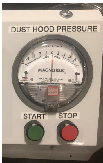
FIGURE 8: DUTHOOD PRESSURE GAUGE ON THE CONSOLE
