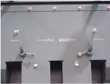
Feed gate valves in open position
