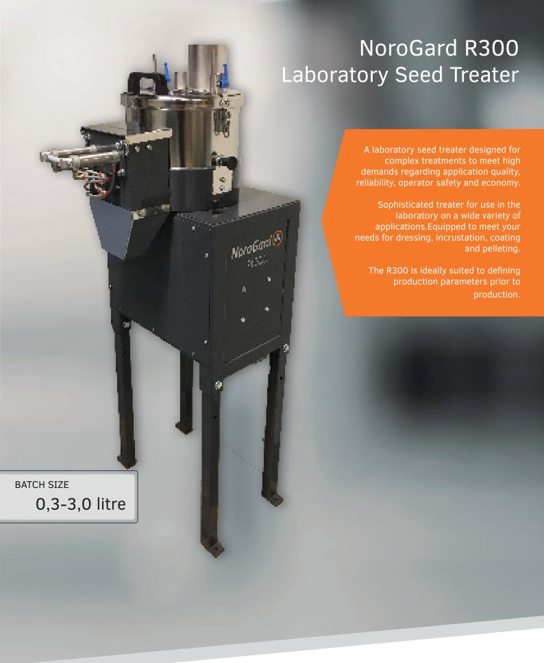
R300 is a laboratory seed treater designed for treating a wide range of seeds with a wide range of products, formulated as liquids, powders, flowables, slurries, gels, etc. It treats seed in batches up to 3000 ml.
