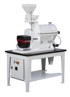
The LA-HO small-scale brushing machine is designed for batch or continuous processing of small volumes of seeds or grain prior to cleaning and grading processes
