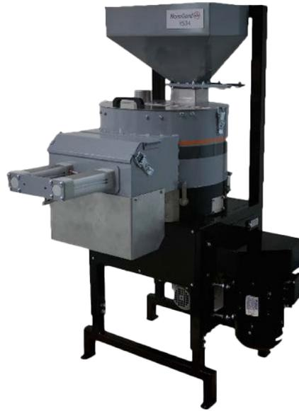
*The R534 batch seed treater is the best choice for a complex treatment such as pelleting, application of separate layers with drying in between, and small seeds like vegetable seeds.*
